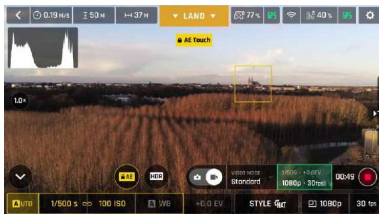
Exposure is locked on a building on the horizon: shutter speed is set at 1/500 s
